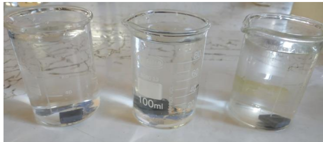
Figure III.16: Protocole du test de corrosion.
