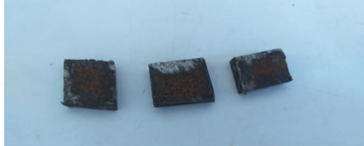
Figure.III.13: Echantillon de l'acier (A 283 grade C).
