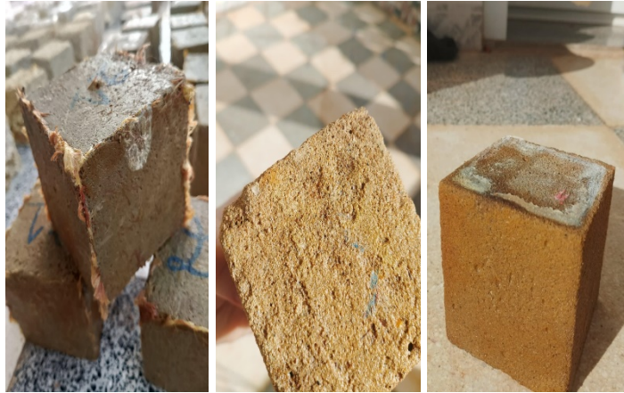
FIGURE II. 21. WEIGHT LOSS --- HYDROCHLORIC ACID (HCL)
