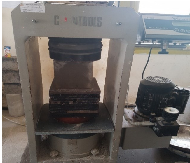
Figure III-7: Essai de compression
