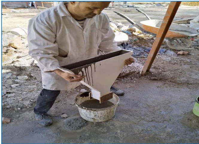
Figure III.11: Essai V funnel
