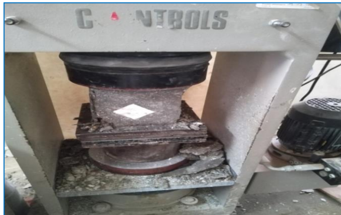
Figure III.12: Essai de compression
