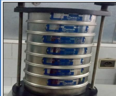
Tamiseuse (Retsch AS 200)
