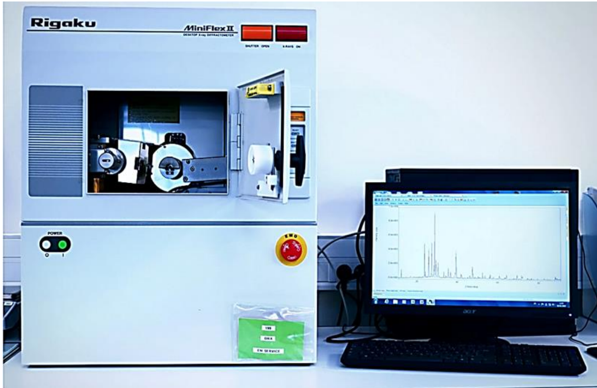
Figure 3. Micro X-Ray Diffraction machine (Original, 2025)
