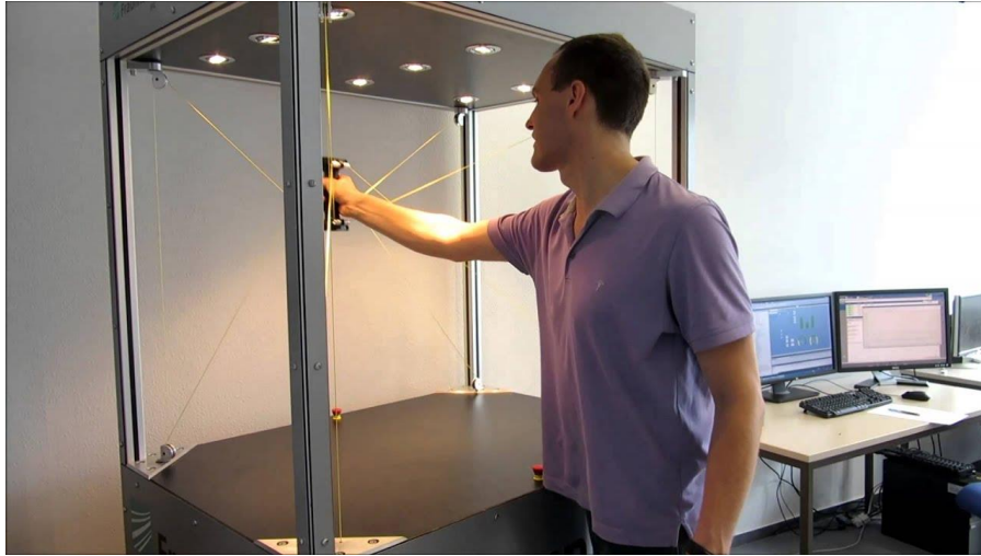
Figure I. 21. IPAnema 3 Mini for haptic interaction ,the Fraunhofer Institute for Manufacturing Engineering and Automation IPA (Matt, 2017 )
