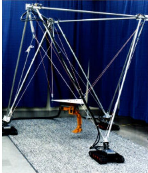
Figure I. 1. RoBoCrane the first parallel robot has been designed ( ROGER BOSTELMAN, 2015 )
