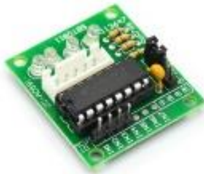
Figure II.36. 28byj-48 motor controller.
