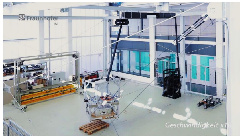
Figure I. 15. Cable robot IPAnema 3 for large-scale handling of collector modules shown. (man, 2020)
