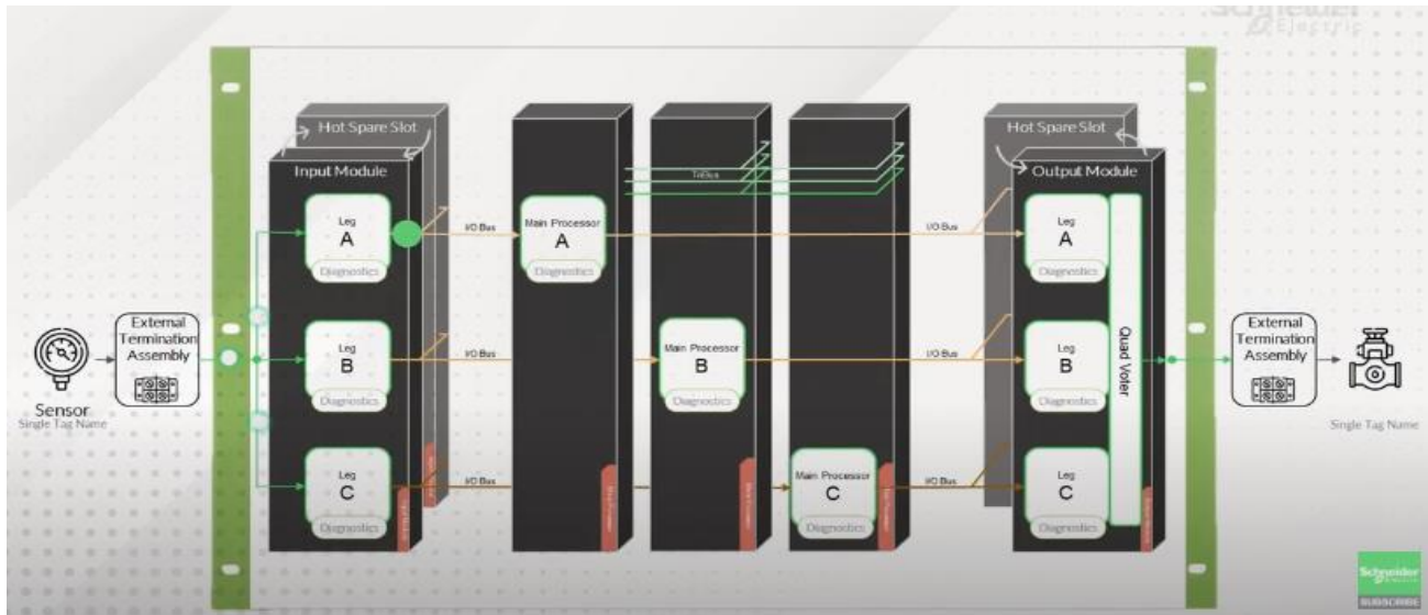
Figure III.7: Architecture Triplée Modulaire Redondante (TMR) [12].
