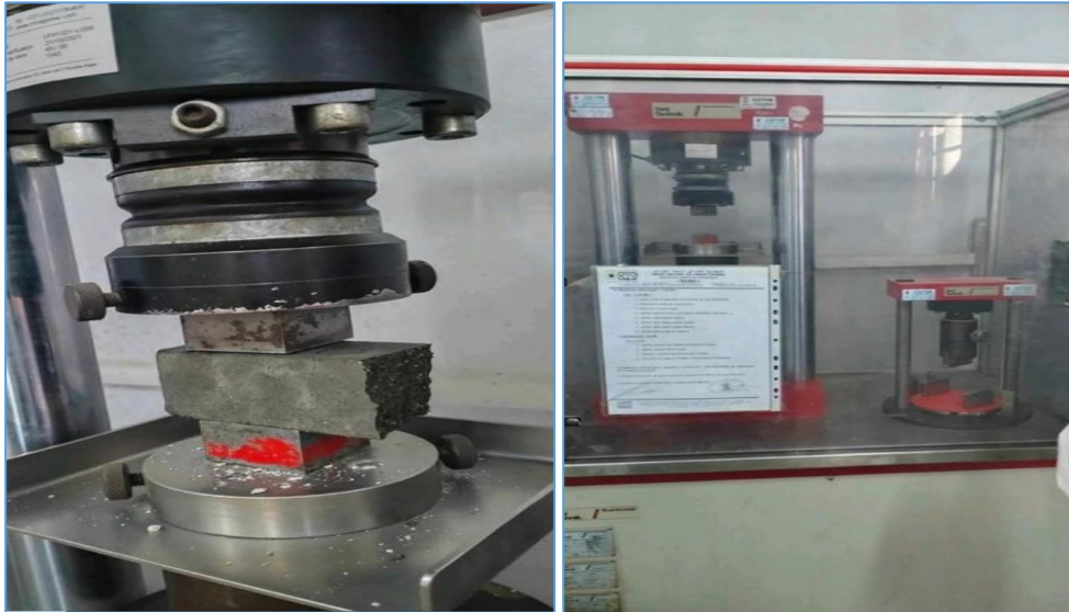
Figure III-12: Presse hydraulique de compression
