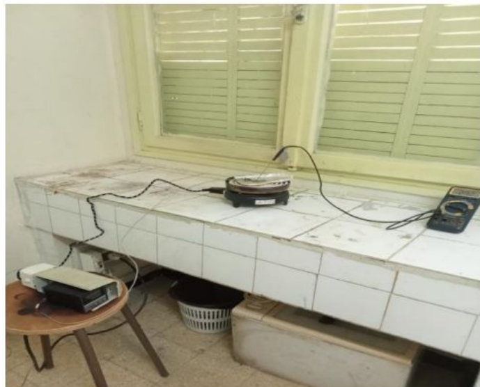
Figure 3.2: Actual mounting of the pyrolysis spray mounted at the LRPCSI laboratory at the University of Skikda.
