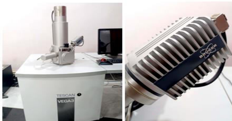
Figure II.32: Appareil du MEB Tescan Vega3.
