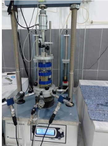
Figure II.20: Appareil triaxial de révolution.
