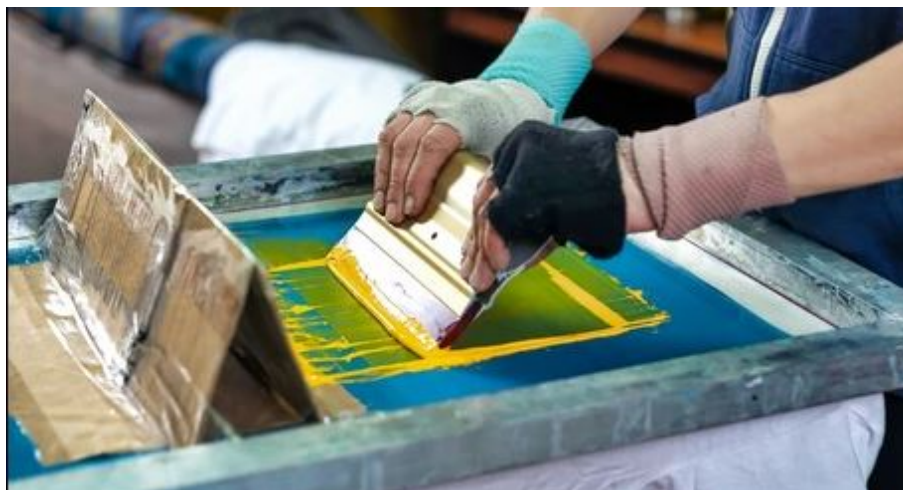
FIGURE 1.5 – Operation de Sérigraphie
