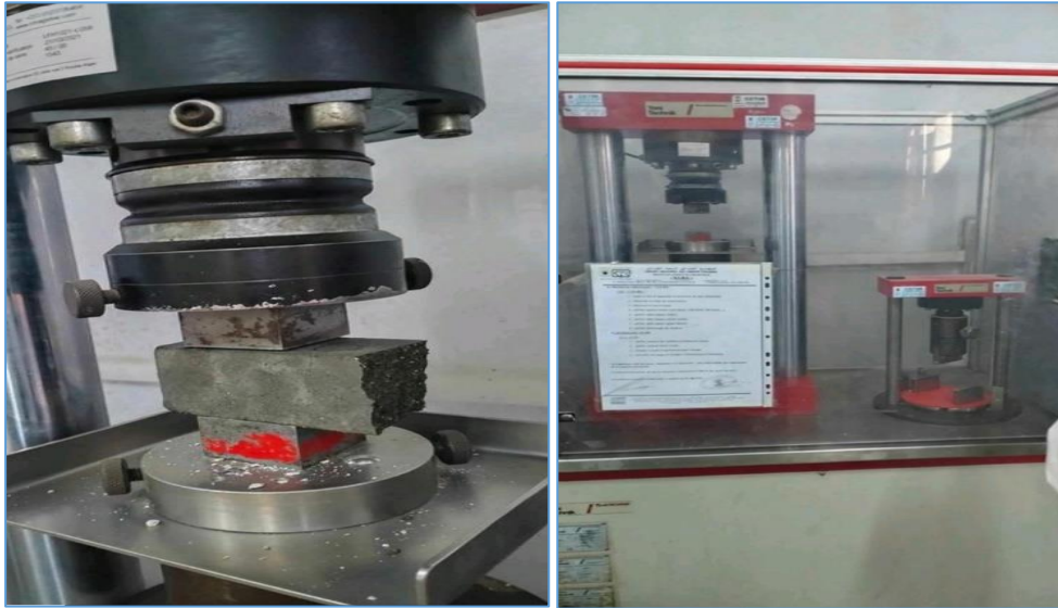
Figure III-12: Presse hydraulique de compression
