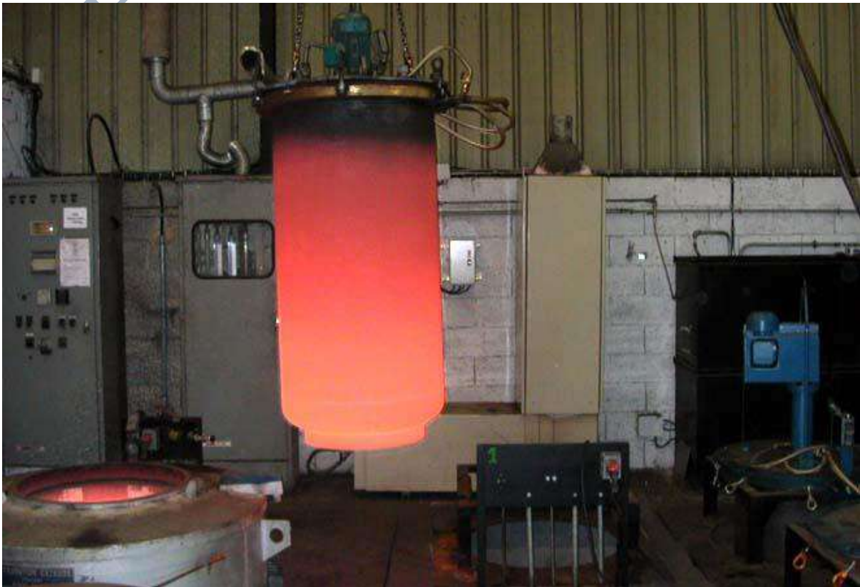
Figure IV 7 Four de nitruration gazeuse
