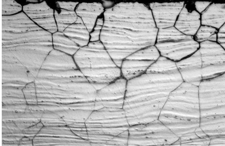
Figure I.3. Schematic representation of intergranular corrosion [9]
