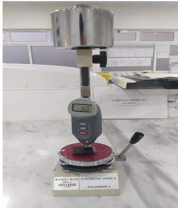
Figure IV.12 : Durometer SHORE D [9].
