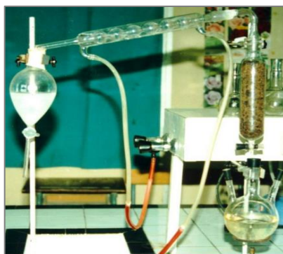
Figure II.6 : Technique de l'hydrodistillation.
