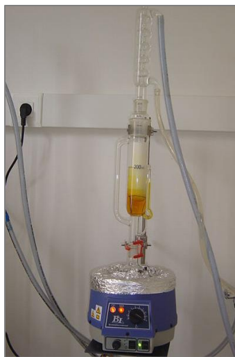
Figure II.7 : Technique de Soxhlet.
