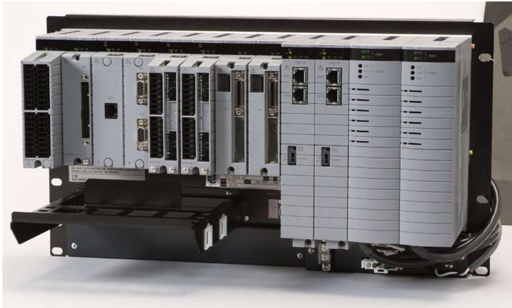
Figure III.3. FCS (Field Control Station).
