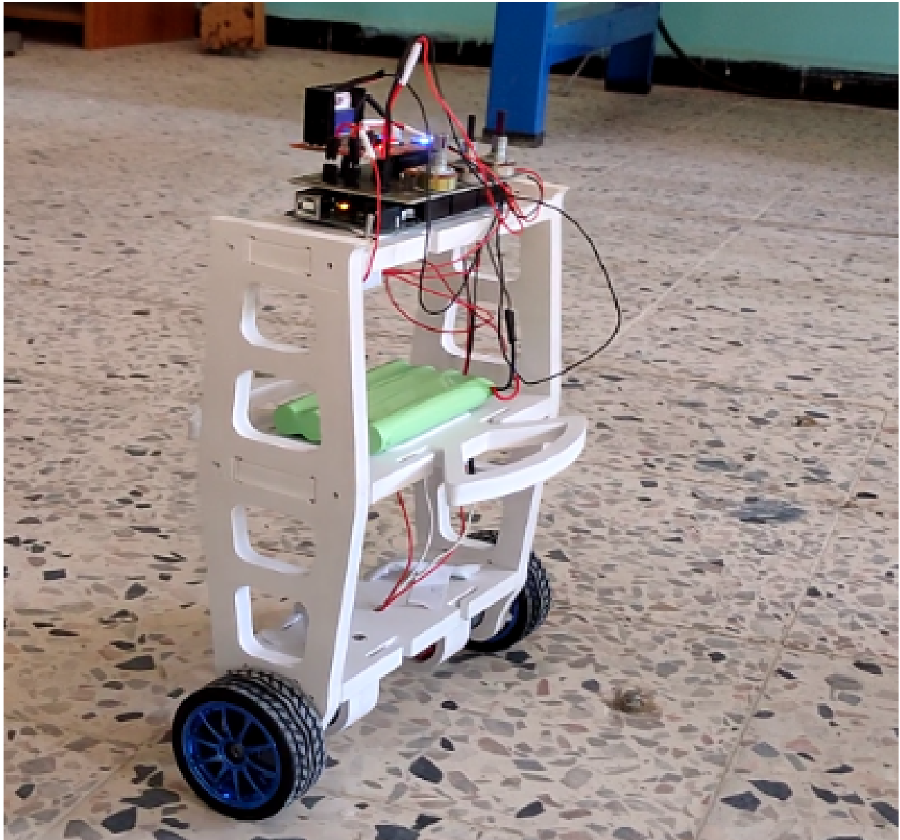
Figure 3.11: The experimental robot achieving a stable equilibrium position after meticulous PID tuning, demonstrating successful balance and control. [13]
