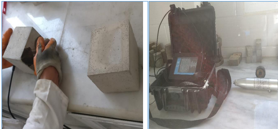
Figure III.17: Essai aux ultrasons en transmission directe
