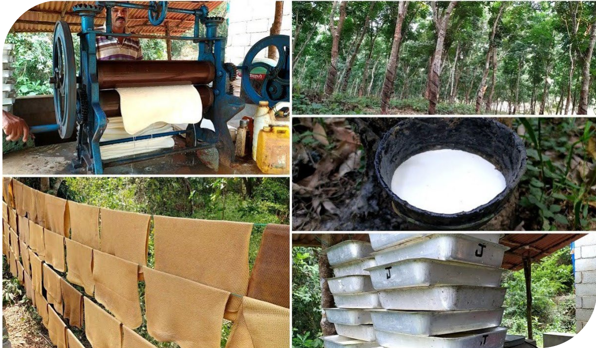
Figure I.5. The process of manufacturing natural rubber.
