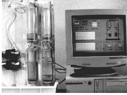
Figure 3.1: The quadruple-tank process shown together with a controller interface running on a PC [82].
