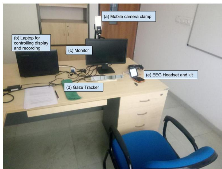
Figure 23 Experimental setup used in the Bag-of-Lies dataset [78].
