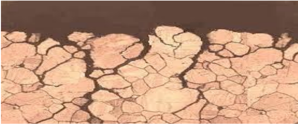
Figure. II.9. Corrosion inter granulaire.
