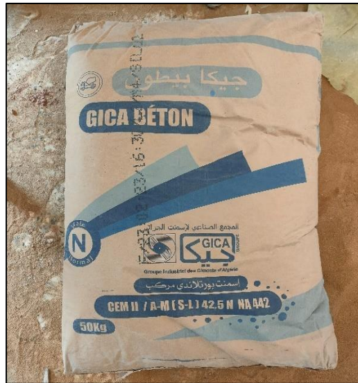
Fig.III.5 Ciment compose CPJ-CEM II 42.5N de Hadjar Essoud
