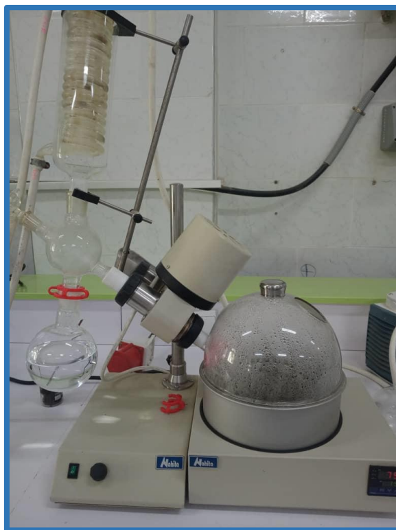
Figure 8. Drying the plant extract in the Rota-vaporator ( Personal photo ).
