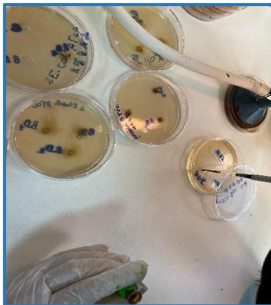
Figure 9. placing the wattman paper discs in agar surface ( Personal photo ).
