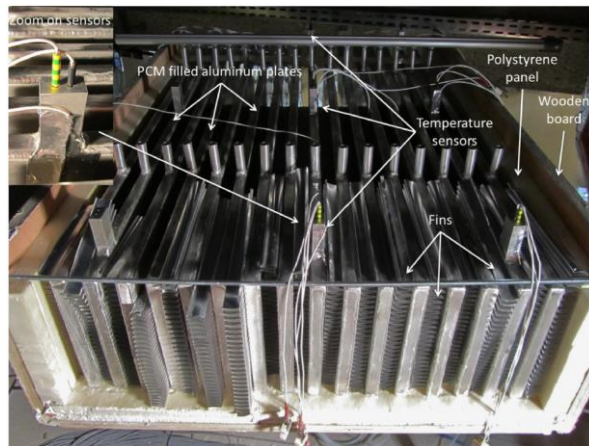
Figure.II.8. The Air-PCM exchanger during fabrication.
