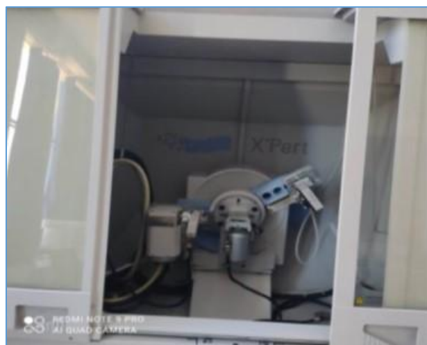
Figure III-24: Diffractomètre DRX (Philips, X'Pert)
