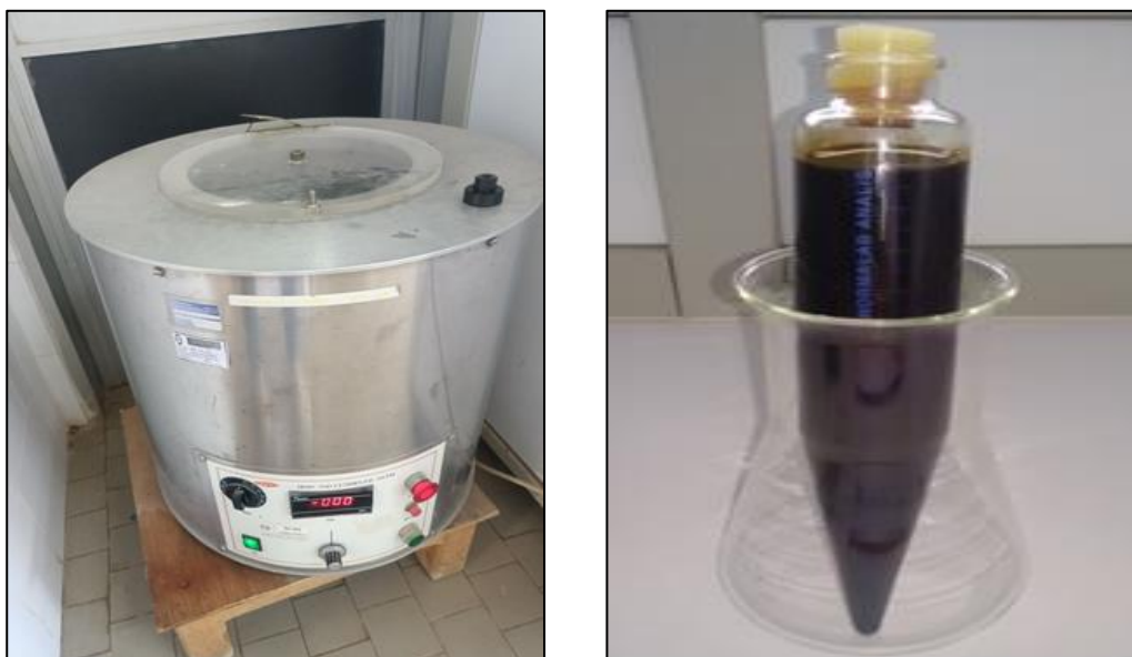
Figure III.12: Centrifugation de l'huile
