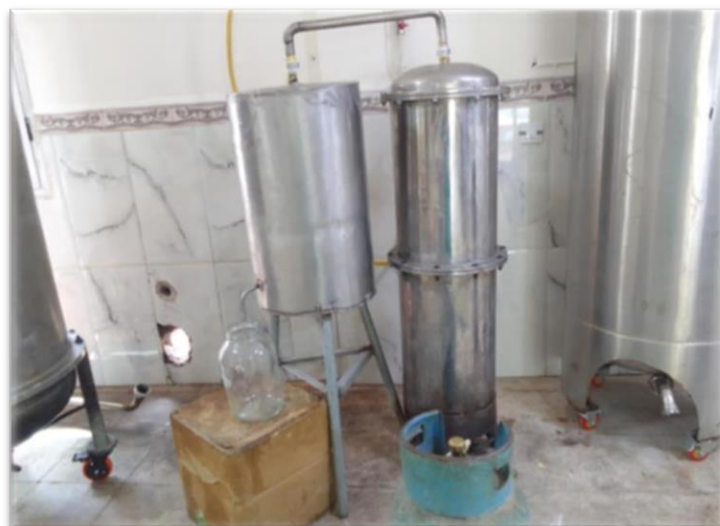
Figure 10: The hydrodistillation technique (Original)
