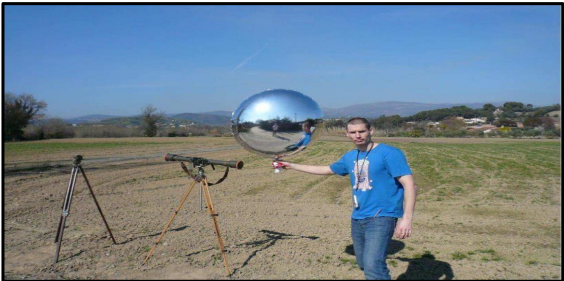
Figure (II.2): CLB is ready to be released on 02/28/2012 around 12 p.m., at La Roquandte-sur- Siagne, at a place called PrésNeufs, view towards the northeast. In the foreground: on the left the theodolite, on the right the rangefinder.
