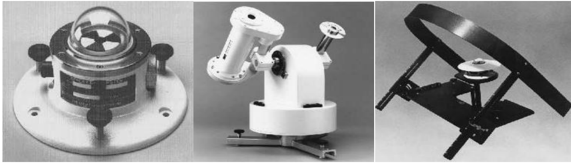
Figure 2. 6 a. Black and white Pyranometer b. Pyrheliometer with tracker c. Pyranometer on shadow band stand
