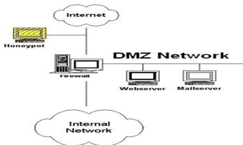
Figure 2.05: Honeypot installé devant le pare-feu.
