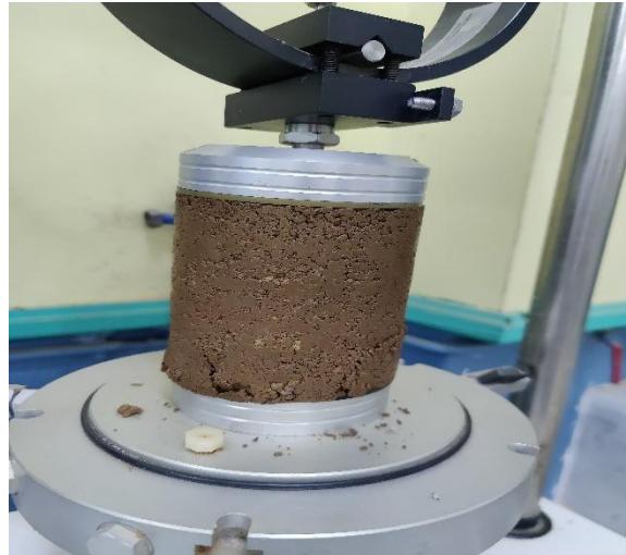
Figure IV.9 : Essai de Compression Simple.
