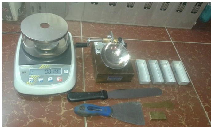
Figure III.8 : Appareillage de Casagrande
