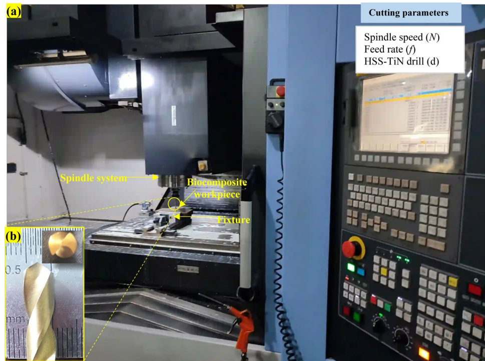
Fig. 1 a Experimental setup for the WF fiber–reinforced epoxy matrix drilling test and b geometry of HSS-TiN drill used in this study
