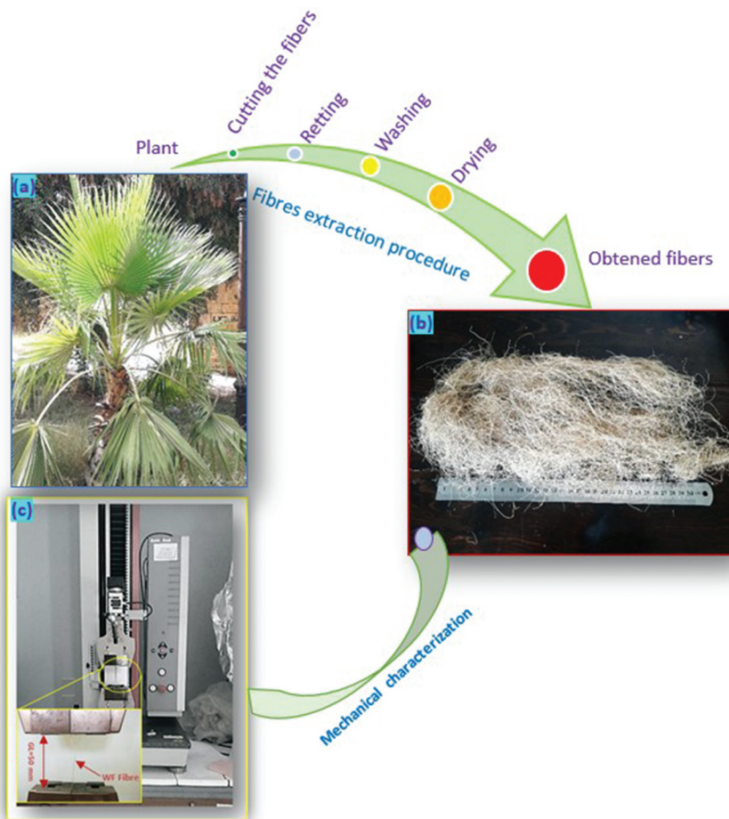
Figure 1. (a) Plant of WF, (b) WF fibers used in this work and (c) equipment to perform the tensile test of single WF fiber.
