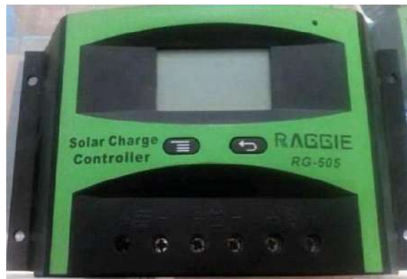
Figure I-14: Charge controller in a PV system.
