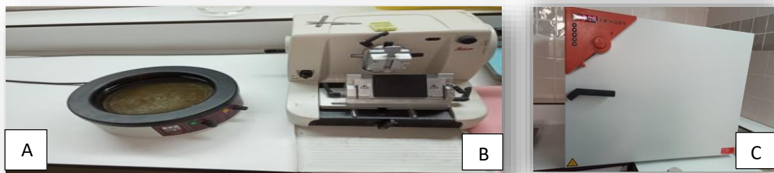
Figure 31 : photo originale, bain marie (A) microtome (B) l'étuve (C)
