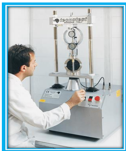
Figure II.12 Application de la compression (Marshall)
