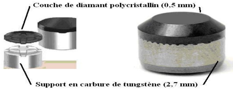
Figure 2.17: Dent (cutter) PDC.
