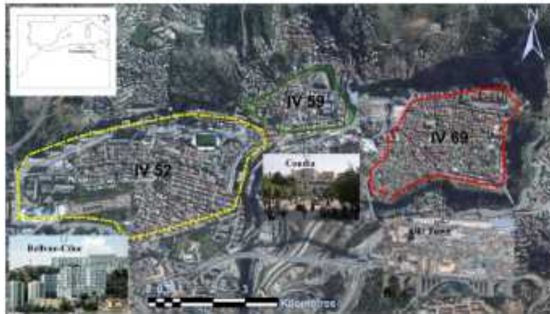
Fig. 14 Example of the boundary of the Bellevue-Cilic area (red-dashed line), mean vulnerability index IV = 52. The boundary of the Coudia area (green-dashed line), mean vulnerability index IV = 59 and the boundary of the Old Town area (yellow-dashed line), mean vulnerability index IV = 69
