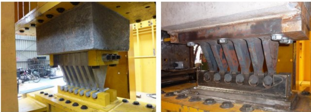
Figure 1.7 Photograph featuring the T-ADAS damper [27]
