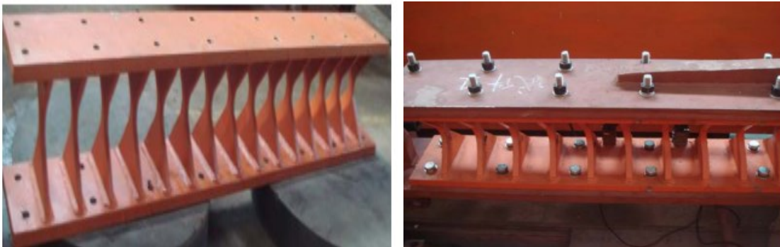
Figure 1.6 Photo of X-ADAS damper [26]
