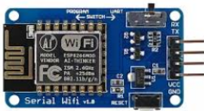
FIGURE 4.5 – Esp8266 / ESP-07 (WIFI)
