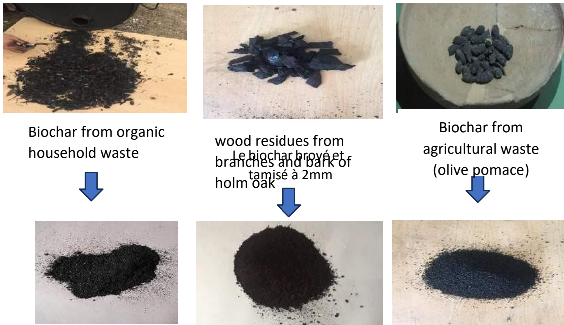
Figure 3 Production of biochar from organic household waste (fruit and vegetable scraps) and agricultural waste (wood residues from branches and bark of holm oak, olive pomace)
