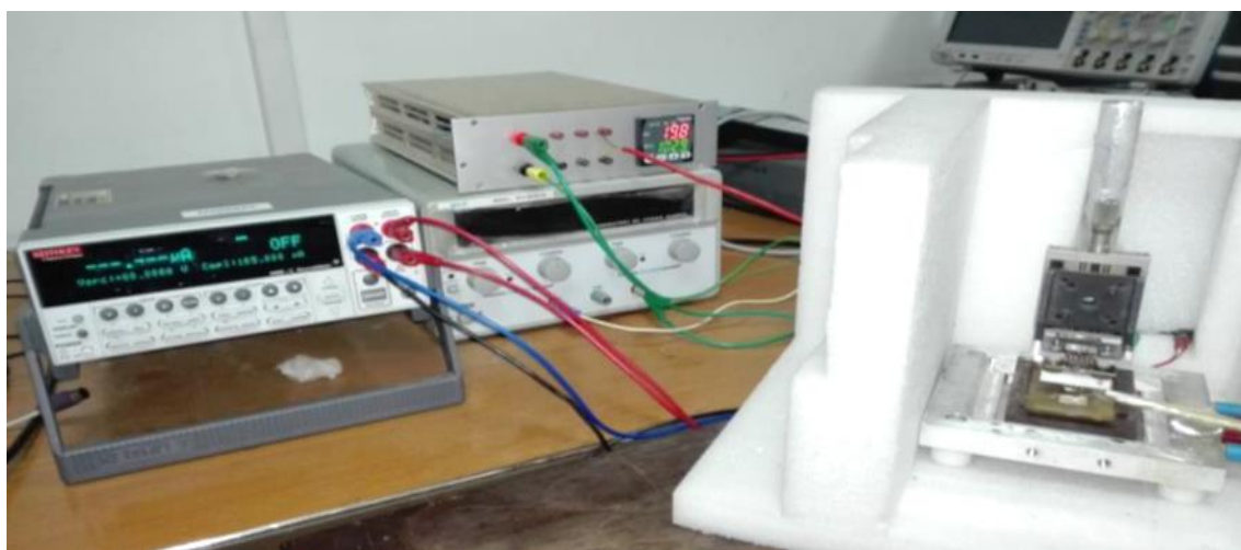
Figure III.7. Photograph of the four-point device.
