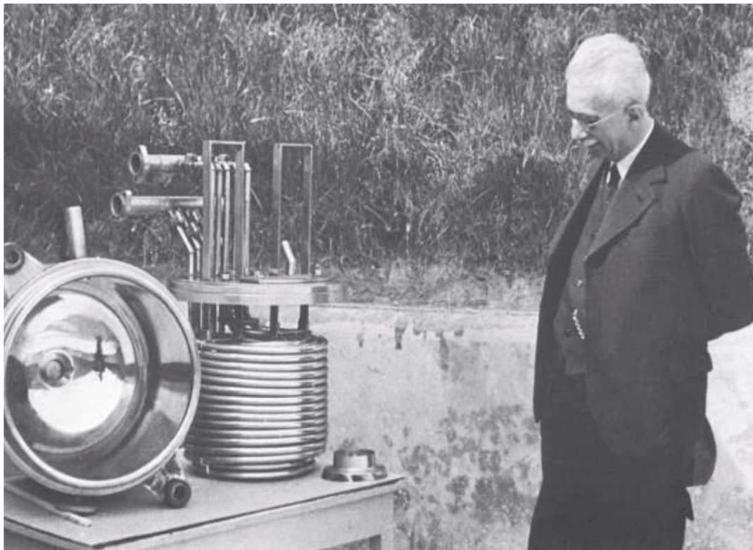
Figure II.2: Continuous nitroglycerine reactor [12]
