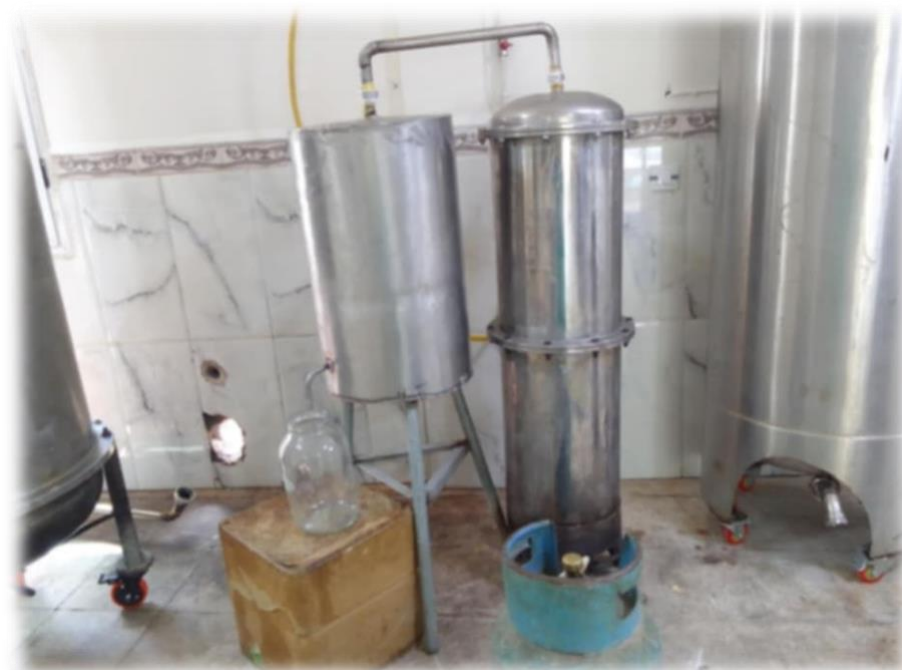
Figure 11: The Hydrodistillation Unit (Original)
