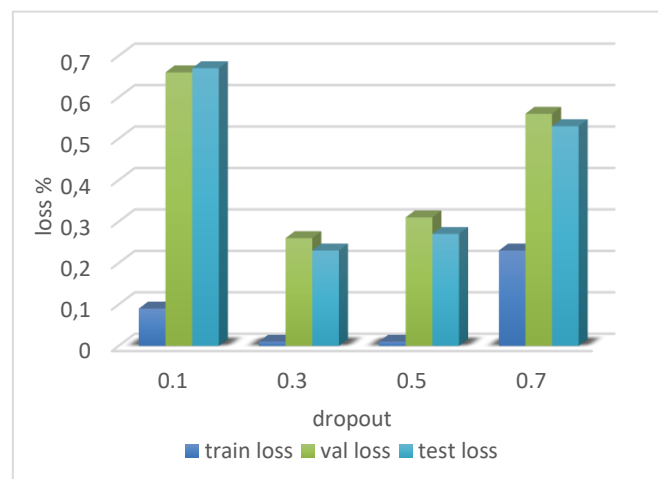
Figure 3. 12 : Loss evaluation of EfficientNet model with Different dropout on PINS-FR dataset.
