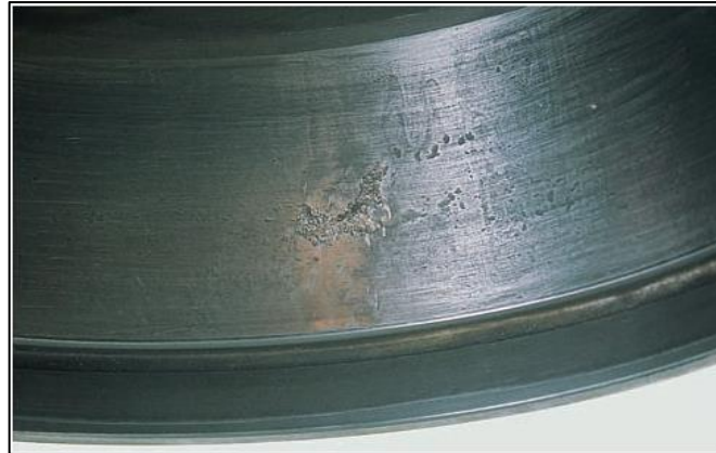
Figure II.24 flaking on the raceway surface causing by electrical damage.
