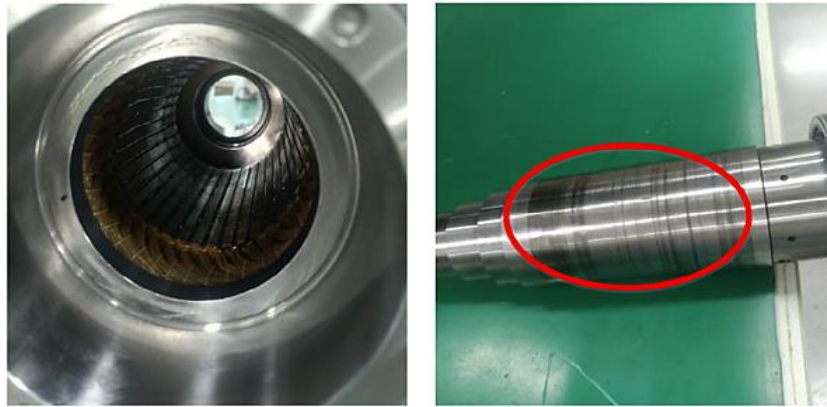
Figure II.14 Rotor-stator contact resulting from an eccentricity defect[93]
