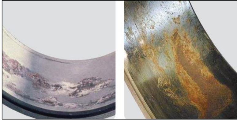
Figure II.25 Fretting corrosion on an inner ring cavity.
