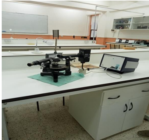
Figure 2. Real image of the goniometer used in our experiment for calculating the angle at the top of the biprism and its deviation
