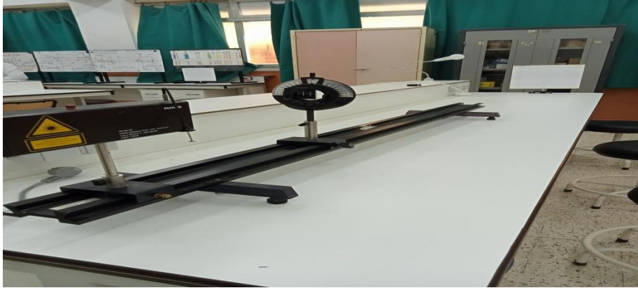
Figure 3. Actual image of the mounting of Young's slits taken in the optical laboratory at Skikda University
