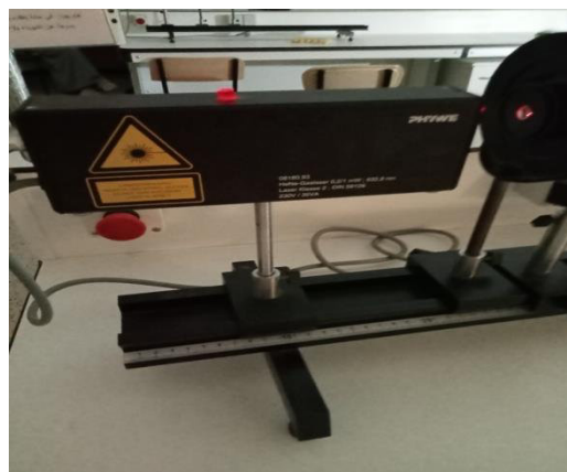
Figure 3. Real image of the He-Ne laser used in our experiment with wavelength \lambda= 632.8 nm and power of 1mwat
