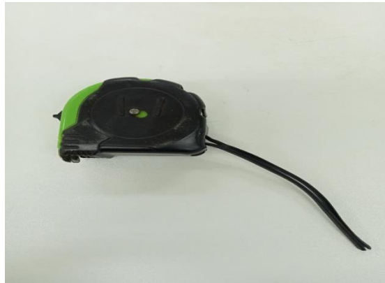
Figure 3. Image of the tool for measuring distances of the order of one metre
