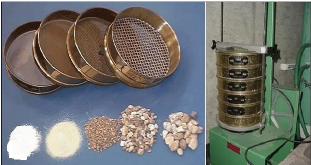
Figure 25. Procedure of grain size analysis of aggregates.
